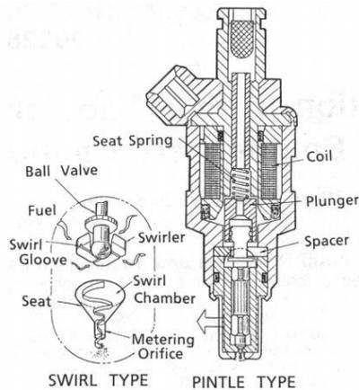
Fig.1 Structure of Injector
