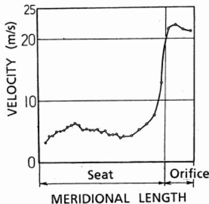
Fig.4 Velocity in Swirl Chamber
