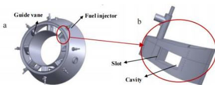
Fig.2. (a)overall schematics of IGC; (b)fuel injector in IGC
