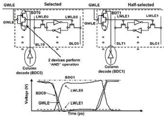
Fig2: SRAM with column Decoupling Logic
