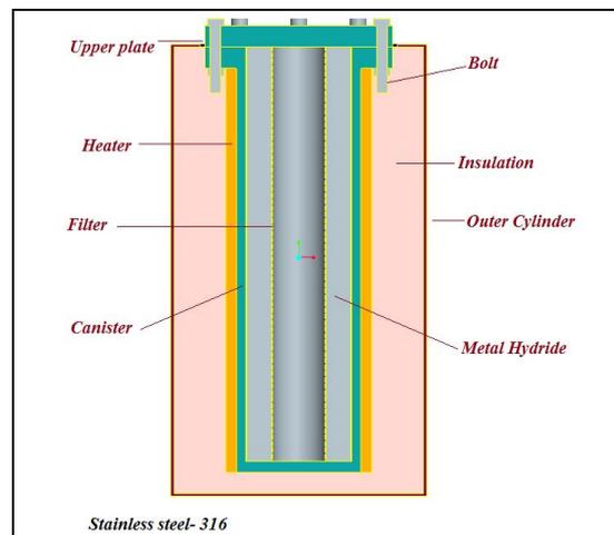
Fig. 2 : Cross-section view of metal hydride reactor;
