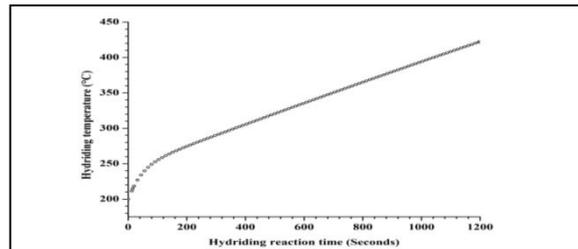
Fig. 5 : Temperature profile during hydriding process
