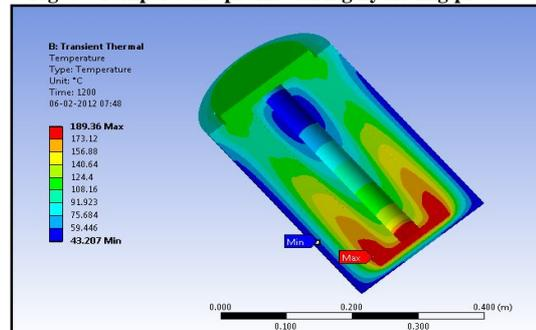
Fig. 6 : Temperature distribution during dehydriding process at time, t=1200 sec, after initiation of dehydriding
