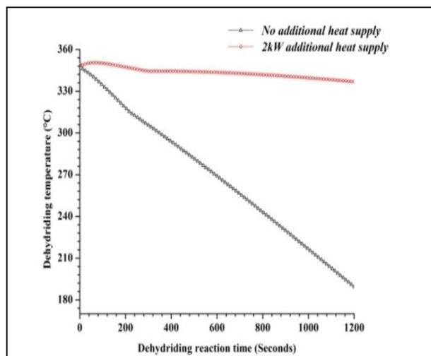
Fig. 7 : Temperature profile during dehydrating process
