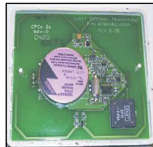
Fig-2-External and internal images of semi passive used for automated toll collection
