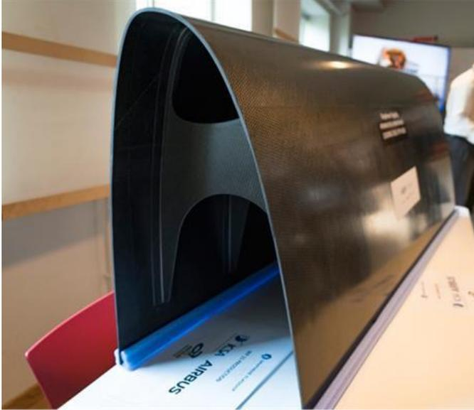
Figure 5. Horizontal tailplane using graphene-based CFRP composite
