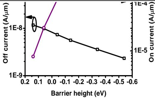
Figure 5: Dependence of ON and OFF currents in a GeOI based SB-FET having channel length of 45 nm.
