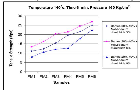
Figure 8 Samples Vs Tensile Strength of fly ash with different percentage of molybdenum disulphide based friction material moulded at temperature 140°C, time 6 min, pressure 160 kg/cm<sup>2</sup>
