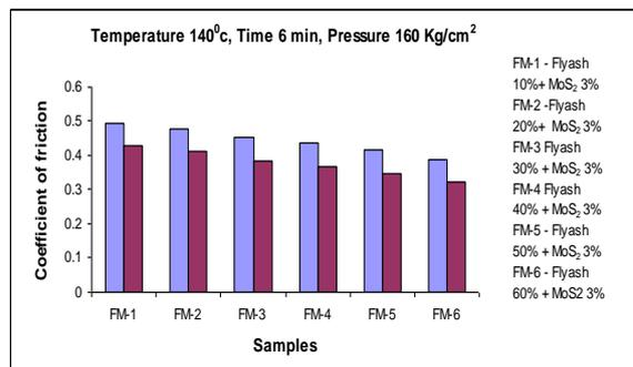
Figure 16 c Coefficient of friction Vs Samples
