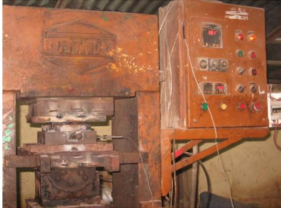
Figure 1 shows conventional compression molding machine used for making friction material.
