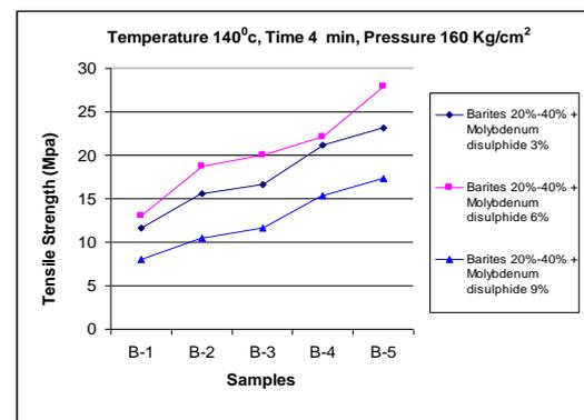
Figure 9 Samples Vs Tensile Strength of barites (without flyash) different percentage of molybdenum disulphide based friction material moulded at temperature 140°C, time 4 min, pressure 160 kg/cm<sup>2</sup>
