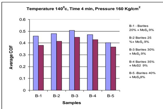
Figure 13 c Samples Vs Average COF of barites (without flyash)
