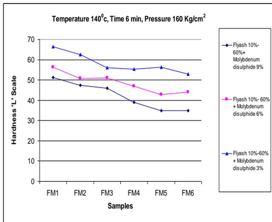
Figure 4 Samples Vs Hardness of fly ash with different percentage of molybdenum disulphide based friction material moulded at temperature 140°C, time 6 min, pressure 160 kg/cm<sup>2</sup>
