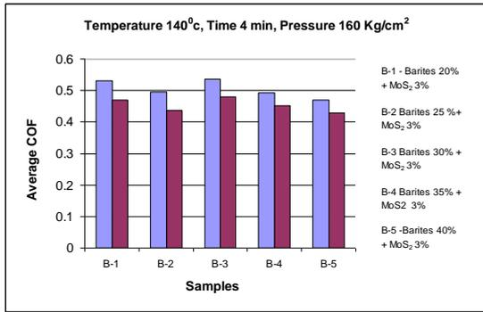
Figure 13a Samples Vs Average COF of barites (without flyash)
