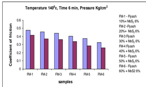
Figure 16 b Coefficient of friction Vs Samples
