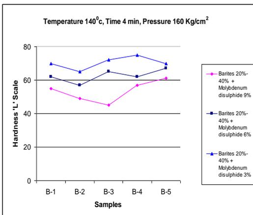
Figure 5 Samples Vs Hardness of barites (without flyash) with different percentage molybdenum disulphide based friction material moulded at temperature 140°C, time 4min, pressure 160 kg/cm<sup>2</sup>
