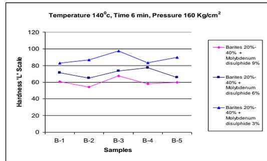
Figure 6 Samples Vs Hardness of barites (Without flyash) with different percentage of molybdenum disulphide based friction material moulded at temperature 140°C, time 6 min, pressure 160 kg/cm<sup>2</sup>
