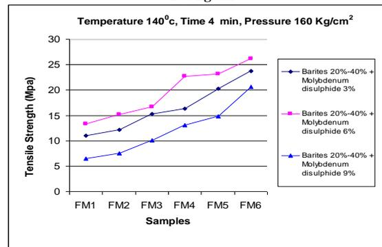
Figure 7 Samples Vs Tensile Strength of fly ash with different percentage of molybdenum disulphide based friction material moulded at temperature 140°C, time 4 min, pressure 160 kg/cm<sup>2</sup>
