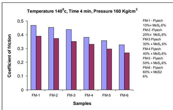
Figure 15 b Coefficient of friction Vs Samples
