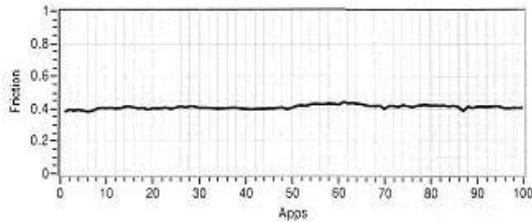
Figure 25 Number of brake application Vs Coefficient of Friction of FM1
