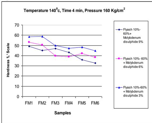
Figure 3 Samples Vs Hardness of fly ash with different percentage of molybdenum disulphide based friction material moulded at temperature 140°C, time 4min, pressure 160 kg/cm<sup>2</sup>
