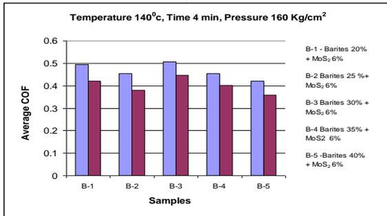
Figure 13 b Samples Vs Average COF of barites (without flyash)
