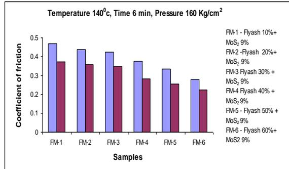
Figure 16 a Coefficient of friction Vs Samples
