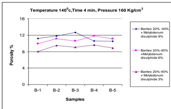
Figure 11 Samples Vs porosity of barites (without flyash) with different percentage of molybdenum disulphide based friction material moulded at temperature 140°C, time 4min, pressure 160 kg/cm<sup>2</sup>
