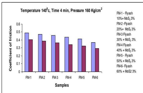
Figure 15 c Coefficient of friction Vs Samples
