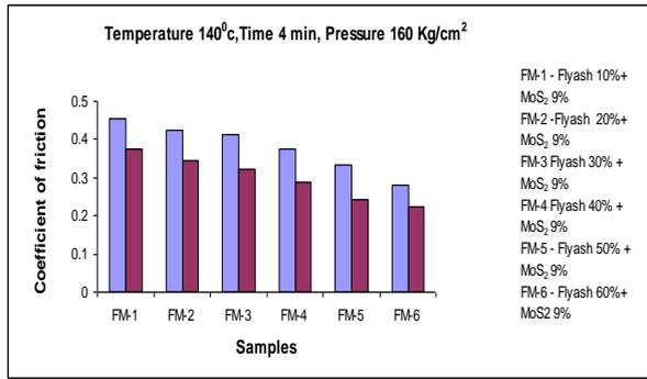
Figure 15 a Coefficient of friction Vs Samples of flyash based molybdenum disulphide friction material molded at temperature 140<sup>0</sup>c, time 4 min, Pressure 160 Kg/cm<sup>2</sup>
