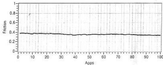
Figure 26 Number of brake application Vs Coefficient of Friction of FM 6
