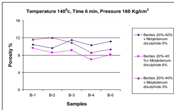
Figure 12 Samples Vs Porosity of barites (without flyash) different percentage of molybdenum disulphide based friction material moulded at temperature 140°C, time 6 min, pressure 160 kg/cm<sup>2</sup>
