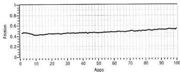
Fig 27 Number of brake application Vs Coefficient of Friction of B-1
