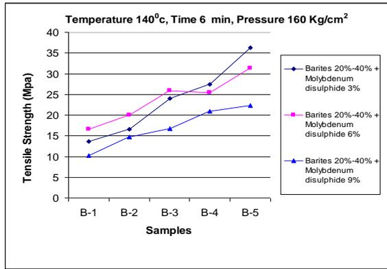
Figure 10 Samples Vs Tensile Strength of barites (without flyash) with 9 %, 6% and 3% molybdenum disulphide based friction material moulded at temperature 140°C, time 6min, pressure 160 kg/cm<sup>2</sup>
