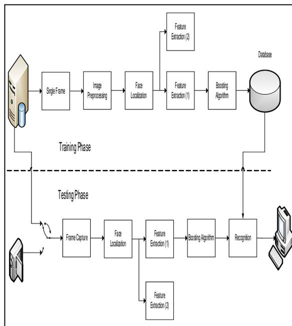
Fig.3 Top level Block Diagram
