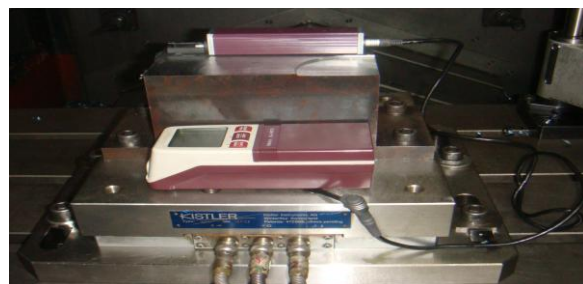
Fig. 7. Surface roughness measurement
