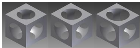
Fig.4 – variation of the base cell for the three models on Spherical Radius (SR)
