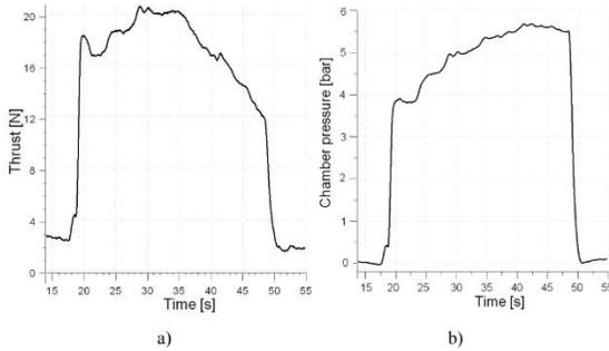
Figure 4. Test results of a hybrid motor test: Thrust (a) and Chamber pressure (b)[1][9]
