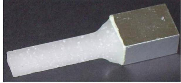
Figure 2. Bubbles on the sample
