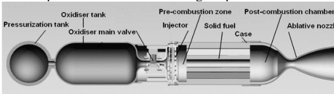
Figure 1. Hybrid rocket motor
