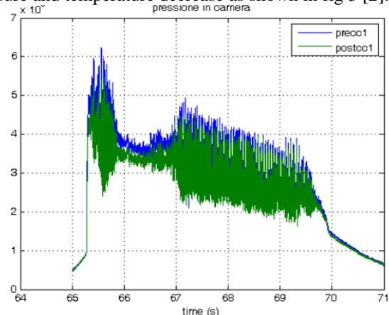
Figure 3. Pre and Post pressure in the combustion chamber
