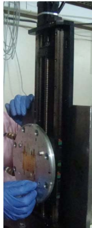
Fig.13. The x-ray mask and PMMA in mounted
