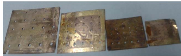
Fig.2. Brass Mask of Basic shapes
