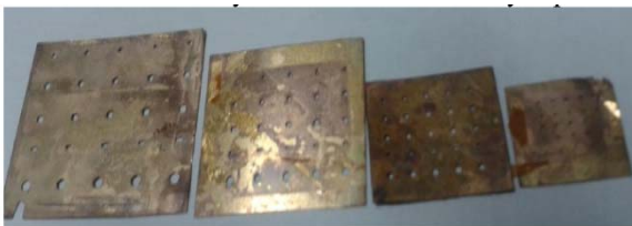
Fig.11. PCM Based X-ray Brass mask of 100µm thickness
