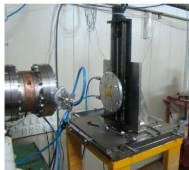
Fig. 14. The x-ray mask and PMMA in mounted on LM guide ways and ready for X-ray Exposure
