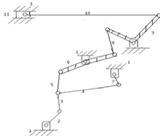
Fig. 3 : Schematic of switch gear mechanism
