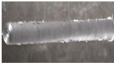
Figure.3. Al-Al weld joint at 900 rpm, speed, 3 D/d ratio
