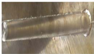
Figure.4. Mg-Mg weld joint at 1120 rpm, 40 mm/min weld speed, 25 mm/min weld speed, 3 D/d ratio
