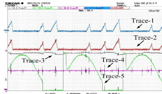
Fig. 10. Experimental results of the converter working in the charging mode when the average bus current is 8.2 A. (1) Recovery current  $i_r$ . (2) Recovery power. (3) Voltage of  $C_0$ . (4) Source input voltage. (5) Voltage between the drain and the source of the MOSFET.
