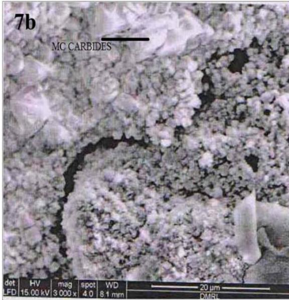
Fig.7: Surface morphology of coated IN 738LC in (a) chloride environment and (b) vanadium environment at 900°C
