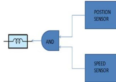
Figure 5 Electronic Circuit
