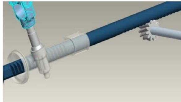
Figure 2 Steering gear box setup
