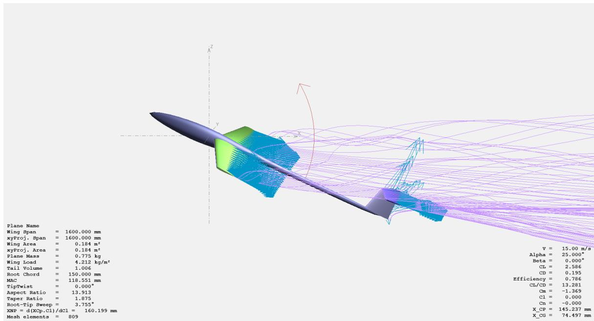
**Figure 5. Aerodynamics of aircraft at 25<sup>0</sup> angle of attack**
