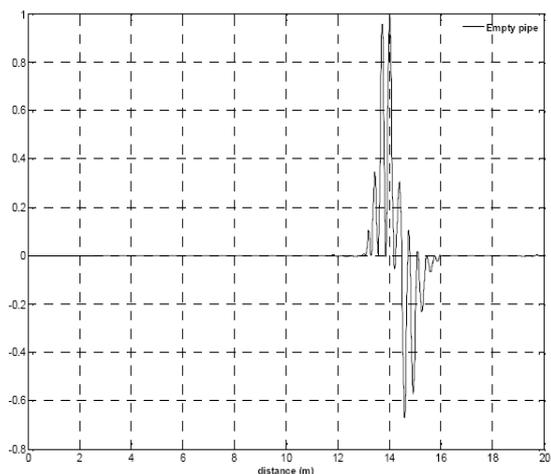
b) Reflection from lateral connection and pipe end of an empty pipe.
