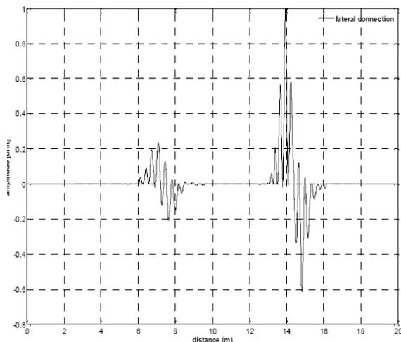
a) Reflection from pipe end of an empty pipe
