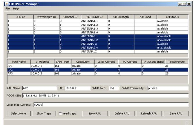
**Figure 7 – Configuration Management GUI**
