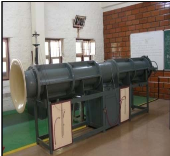
Fig: 3 Side view of Ducted Axial Fan Rig
