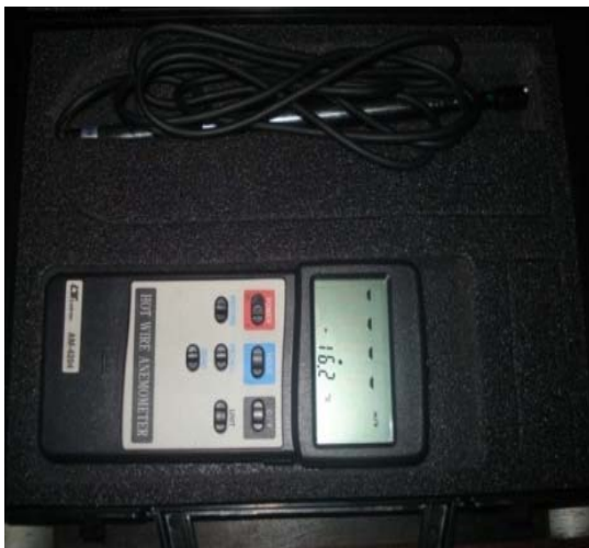
Fig: 5 Velocity Measurement – Hot Wire Anemometer
