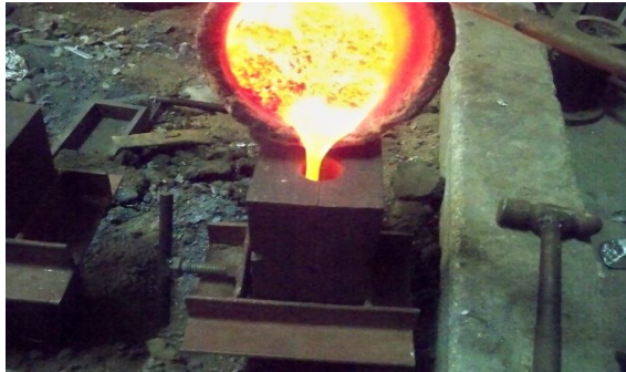
Fig 5: pouring molten metal into mould box
