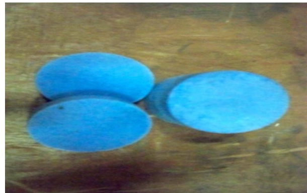
Fig 3: degasifier (exo-chloro ethane)
