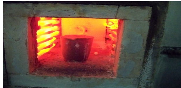
Fig 2: loading al 7075 in to furnaces with crucible
