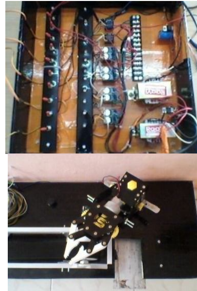
Fig. 3 : Relay Panel And Conveyor With Robotic Arm
