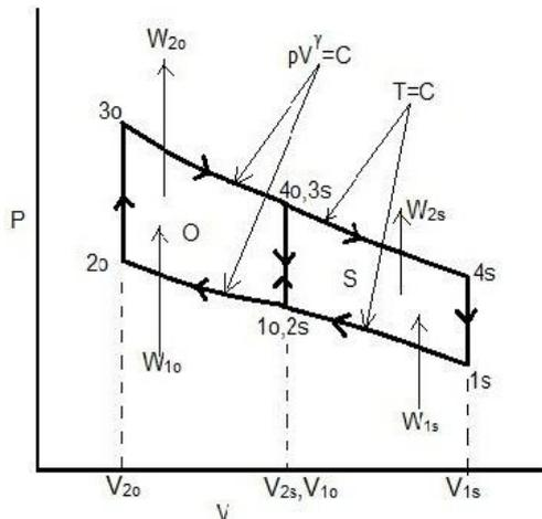
**Fig. 10: p-V diagram of Dual Cycle**
