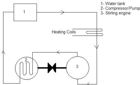
**Fig. 8: Layout of Closed Water Cycle**
