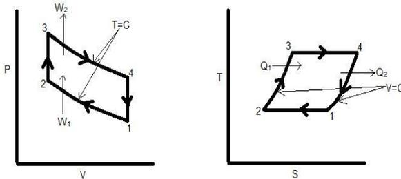
**Fig. 5: Stirling Cycle**
