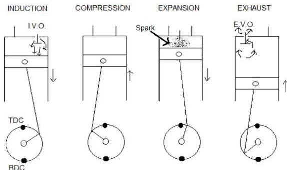
Fig. 1: Four strokes of an IC Engine
