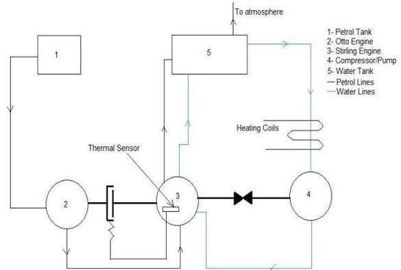
**Fig. 6: Working Layout of Concept ECO-TWINGINE**
