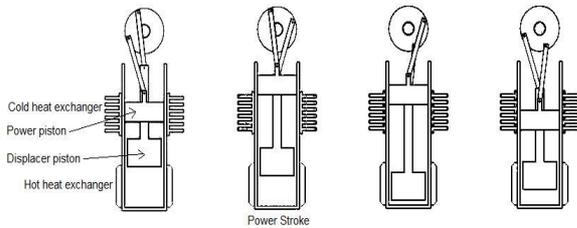
**Fig. 4: Working of a Stirling Engine**
