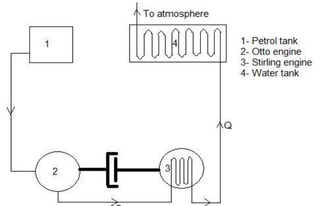
**Fig. 7: Layout of Open Petrol Cycle**
