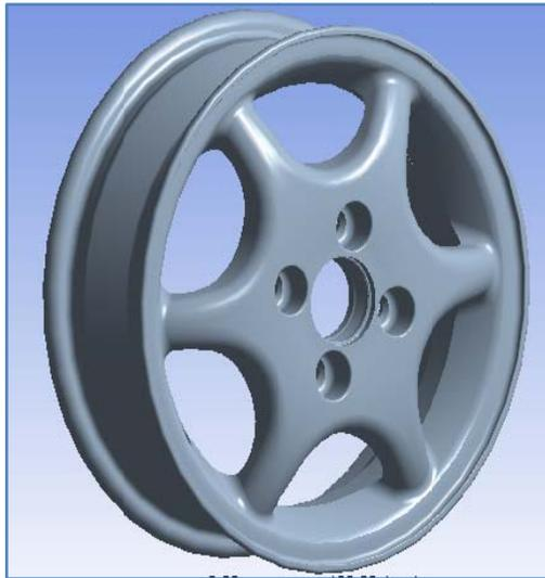
Figure 2. 3D Model of Aluminum alloy wheel
