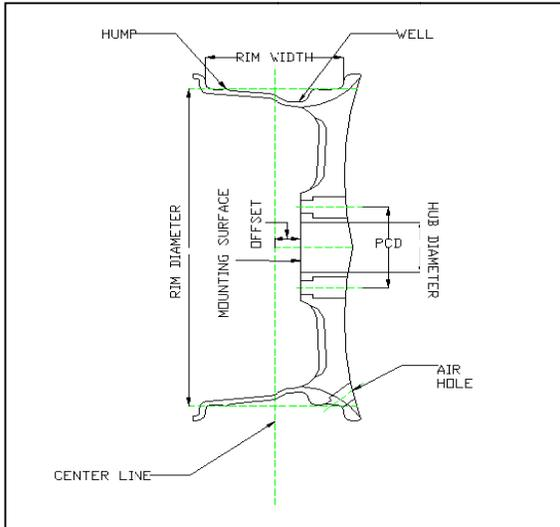
Figure 1. 2D Diagram of aluminum wheel
