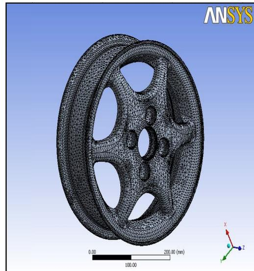
Figure 3. Meshing of alloy wheel
