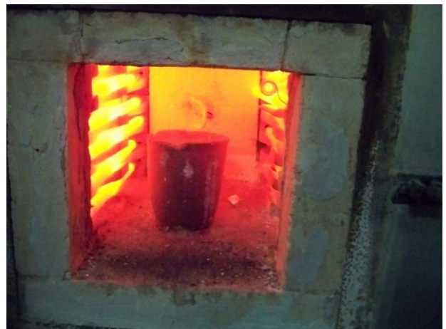
Fig 2: Loading Al 7075 in to Furnaces With Crucible
