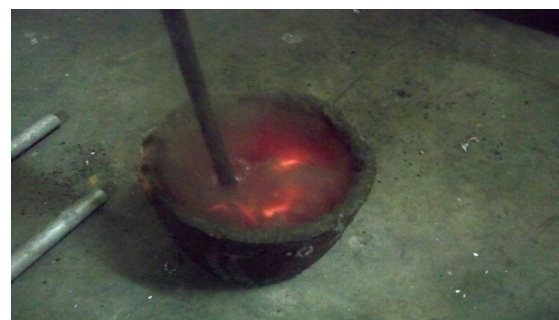
Fig 4: Stirring After Adding Reinforcements
