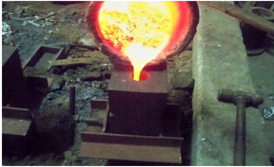
Fig 5: Pouring Molten Metal Into Mould Box
