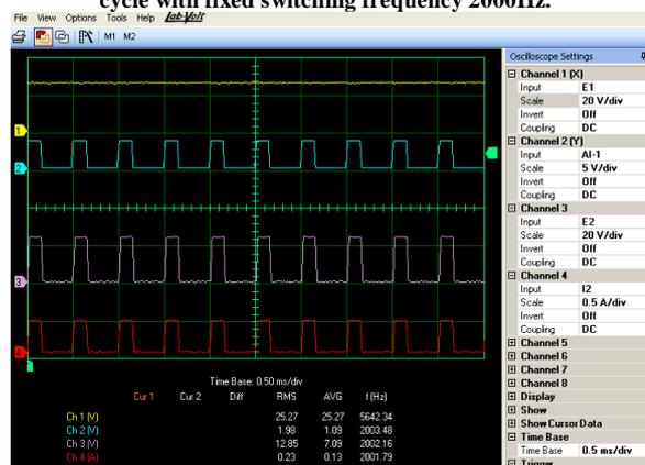
**Figure 6. Waveform of output voltage and output current for low side switching configuration of buck converter at 30% duty cycle with fixed switching frequency 2000Hz.**
