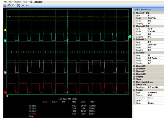
**Figure 10. Waveform of output voltage and output current for low side switching configuration of buck converter at 70% duty cycle with fixed switching frequency 2000Hz.**
