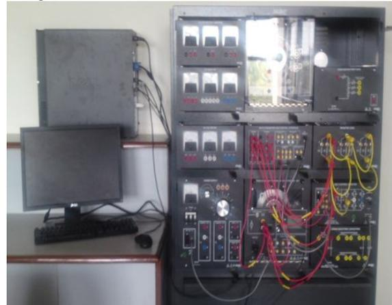
Figure 4: Experimental setup of buck converter.
