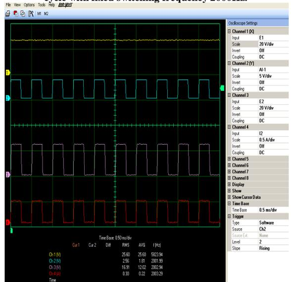
**Figure 8. Waveform of output voltage and output current for low side switching configuration of buck converter at 50% duty cycle with fixed switching frequency 2000Hz.**
