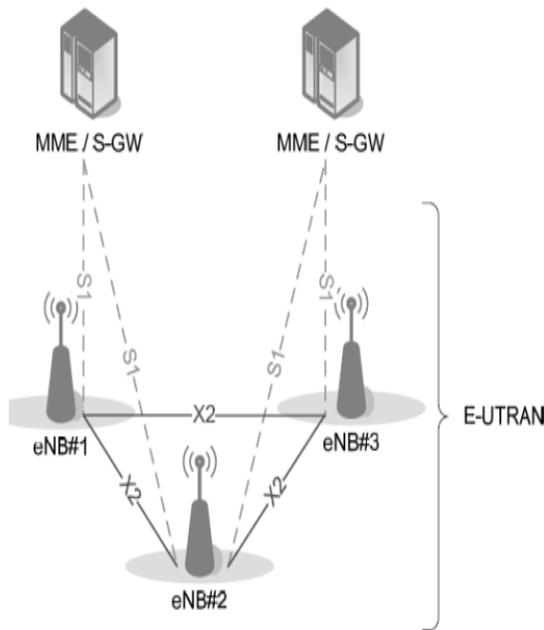
Figure 3: LTE (release 8) architecture
