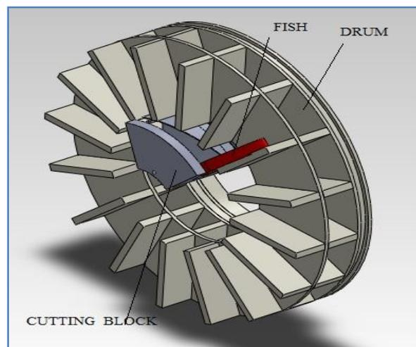
Fig.6 : Cross section of the drum with the fish being cut
