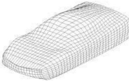
Figure 6: The basic geometry for the analysis of the 360 Modena
