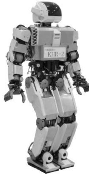
**Figure-2 (KHR-2 Biped humanoid robot)**
