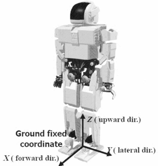
**Figure-5 (3D coordinate system of biped robot)**
