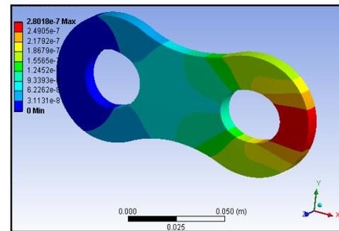
Fig. 10 : Deformation in link
