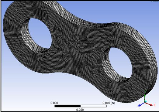
Fig. 8 : Shows the meshed model with 1mm element size
