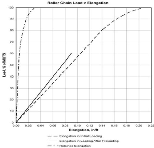
Fig. 4 : Standard roller chain elongates as a tensile load is applied
