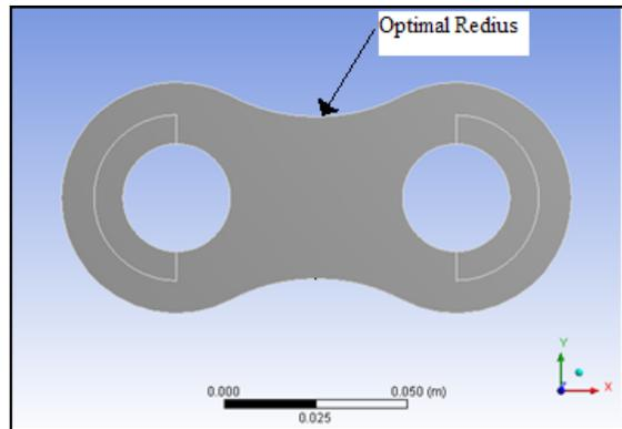
Fig. 7 : Shows the optimizing radial distance
