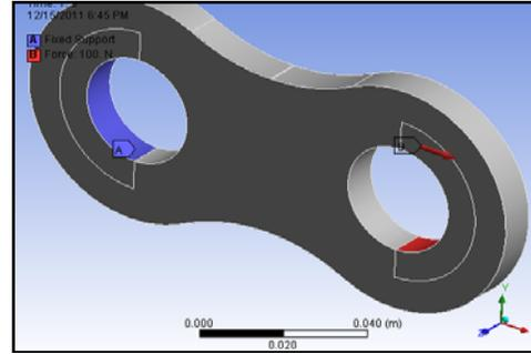
Fig. 9 : Applied boundary conditions
