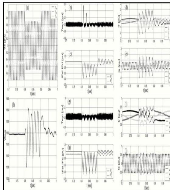
Fig. 2 Simulation comparison of DFIM behavior, without (\*) and with (\*\*) proposed reference generation. (a) Stator voltage. (b) Torque\*. (c) Stator and rotor fluxes\*. (d) Rotor currents\*. (e) Stator currents\*. (f) DC bus voltage\*\*. (g) Torque\*\*. (h) Stator and rotor fluxes\*\*. (i) Rotor currents\*\*. (j) Stator currents\*\*
