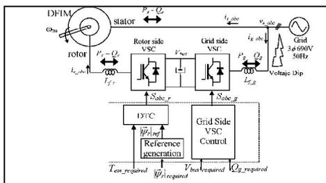
Fig.1. Wind energy generation system based on the DFIM
