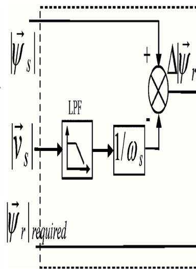
**Fig. 3 Rotor flux reference generation strategy**
