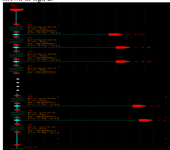
Fig. 2: Resistor string for proposed flash ADC.
