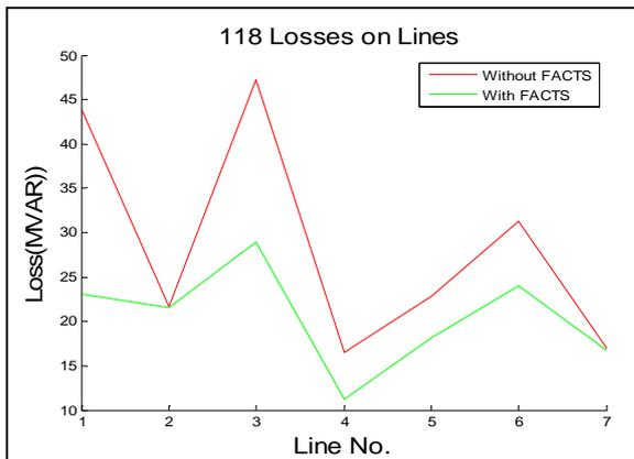
Figure 6 118 Bus IEEE System Performance Before and After Placing STATCOM
