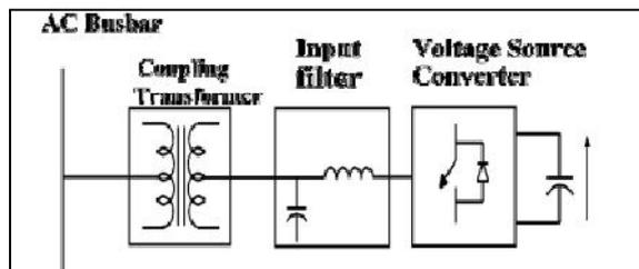
Figure 2. Connection of STATCOM to AC Bus Bar
