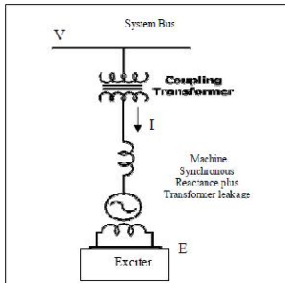
Figure 3 Reactive power generation by a synchronous compensator
