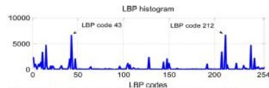
Fig. 11. LBP histogram  $h_{LBP}(l), 0 \leq l \leq 254$  of a signature from GPD5960GraySignature corpus. Codes 43 and 212 corresponds to edges structures orientated North West.
