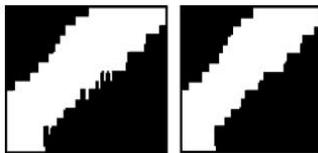
Fig. 4. Eliminating hair-like noise from signature strokes. (Left) signature stroke detail of  $I_{bw}(x, y)$  with noise. (right) Same signature stroke detail of  $I_{NR}(x, y)$  without noise.
