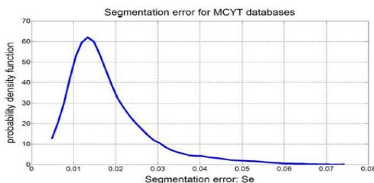
Fig. 8. Distribution of automatic segmentation error  $Se$ .
