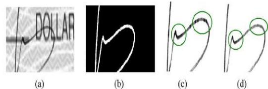
Fig. 6. Segmentation procedure. Details of (a) original image  $I_D(x, y)$  with 256 gray levels, (b) binarized signature  $I_{NR}(x, y)$ , (c) segmented signature  $I_{GD1}(x, y)$  with gray level distortion, (d) segmented signature  $I_G(x, y)$  without gray level distortion. Circles identify some gray level differences.
