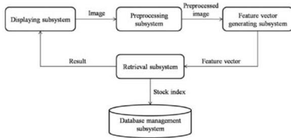
Fig. 1. The global structure of the system.
