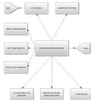
Fig. 1: Block diagram of humanoid control system.
