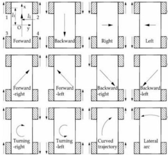
Fig. 7: Robot motion according to the direction and angular speed of the wheels
