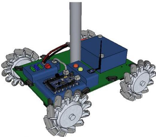
Fig. 8 : Design of Mecanum drive chassis with sensors
