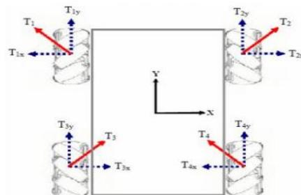
Fig. 6 : Force vectors created by Mecanum wheel.
