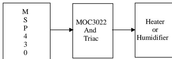
Figure10. Interfacing of Triac triggering circuit with MSP430
