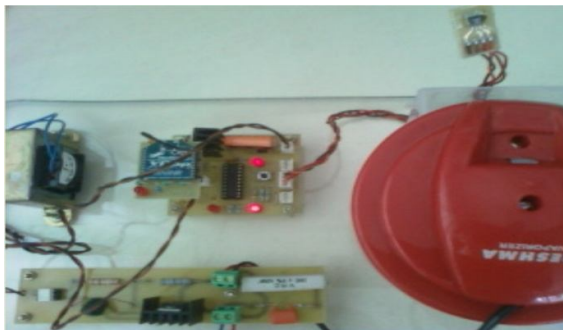
Figure15. Interfacing of sensor SHT11, zigbee and control unit with MSP430
