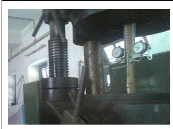
Figure 2. Tension Test on Bamboo Splint
