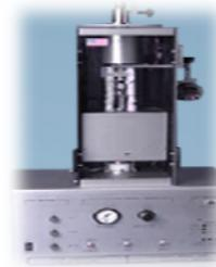
Guarded heat flow meter test method was used to measure the thermal conductivity of Typha angustifolia fiber reinforced polyester composites using an instrument Unitherm™ Model 2022 in accordance with ASTM-E1530. The sample of size 50 mm in diameter and 10 mm in thickness is placed in between two polished surfaces and a pneumatic pressure of 70 kPa were applied on the top portion of the stack.
