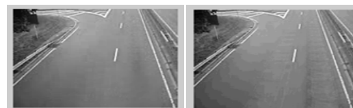
(A) ORIGINAL BACKGROUND (B) GHOST OF MOVING VEHICLES FIG 1: GHOST OF MOVING VEHICLE EFFECT ON BACKGROUND FRAME IMAGE SEQUENCES.
