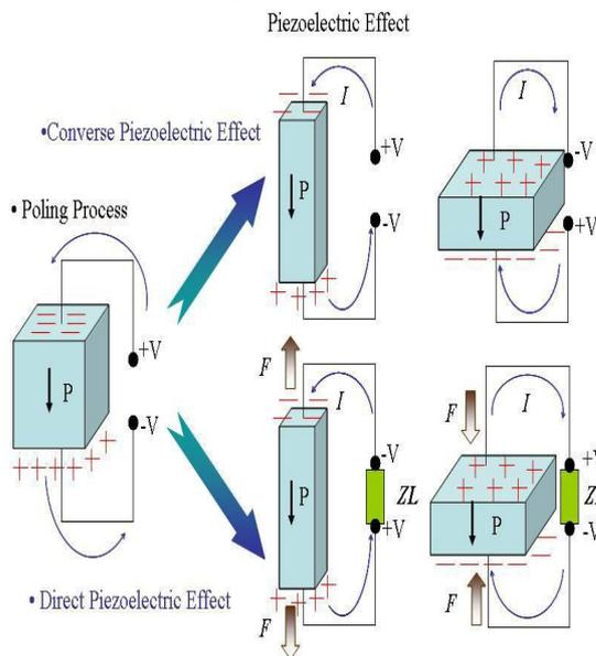
Fig.10 Piezoelectric effect
