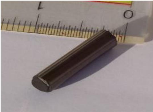
Fig 6 A small rod of glassy carbon
