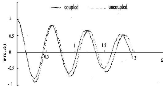
Fig. 2 The decay of vibration amplitude in coupled field with large initial displacement
