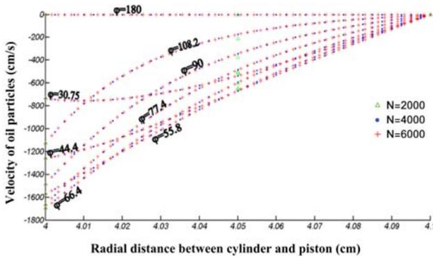
Figure 5. Velocity profiles for downward motion of piston (angle  $\phi$  is in degree)
