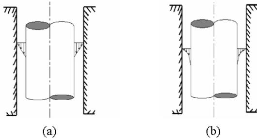
Figure 1. (a) linear and (b) nonlinear oil velocity profiles between piston and cylinder
