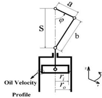
Figure 2. Schematic of a crank and slider mechanism and notations
