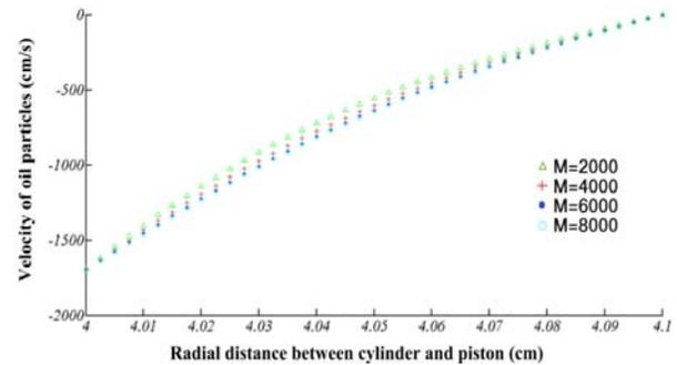
Figure 7. Grid independency of the results in radial direction
