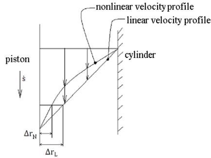
Figure 8. Comparison of the results of linear and nonlinear oil velocity profiles
