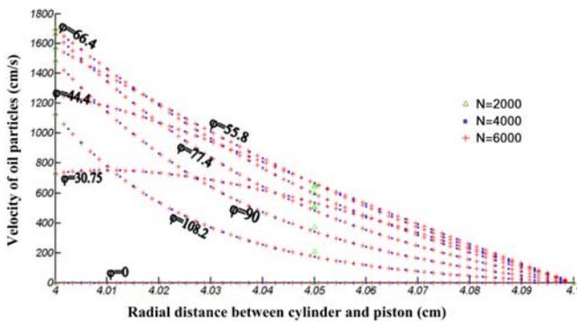
Figure 6. Velocity profiles for upward motion of piston (angle  $\phi$  is in degree)
