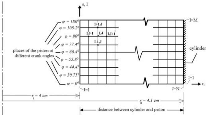
Figure 3. Coordinates and grids in the domain between piston and cylinder
