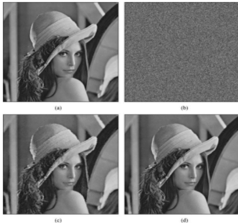
Fig.5 . (a) Original image Lena, (b) its encrypted version, (c) the medium reconstructed image from compressed data with PSNR 39.7dB, and (d) the final reconstructed image with PSNR 43.7dB.
