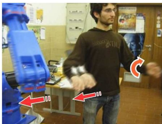
Fig. 9. The user makes a gesture and immediately, the robot starts to move in the same direction of his/her right arm.
