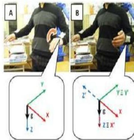
Fig. 8. Postures performed by the user left arm. A - Robot stopped. B - The robot starts the movement.
