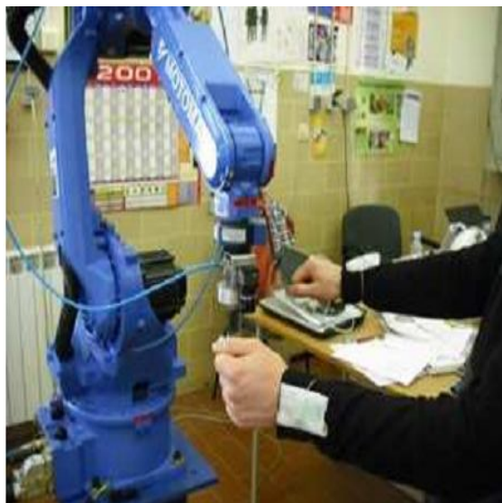
Fig. 1. Industrial robot MOTOMAN HP6 controlled by arm gestures and postures.
