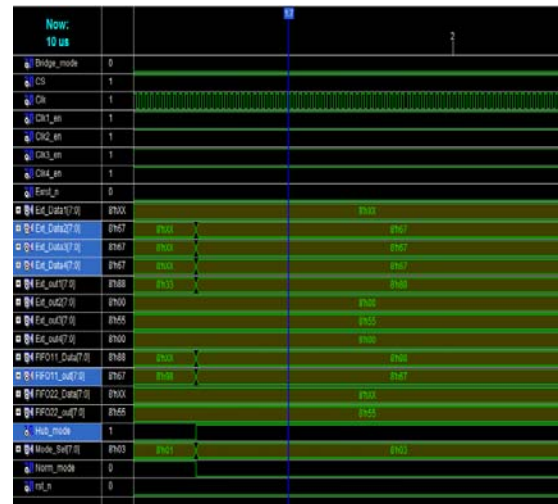
Fig. 4 : Controller Waveform in Hub Mode
