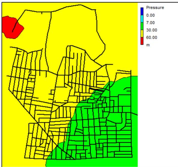
Figure 4: Contour Plot of Pressure of Water Distribution System for Hanumanth Nagar Ward
