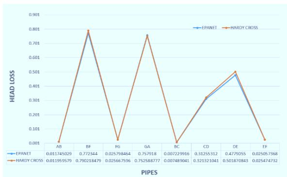
Figure 9: Comparison of EPANET and Hardy Cross Values with respect to Head Loss
