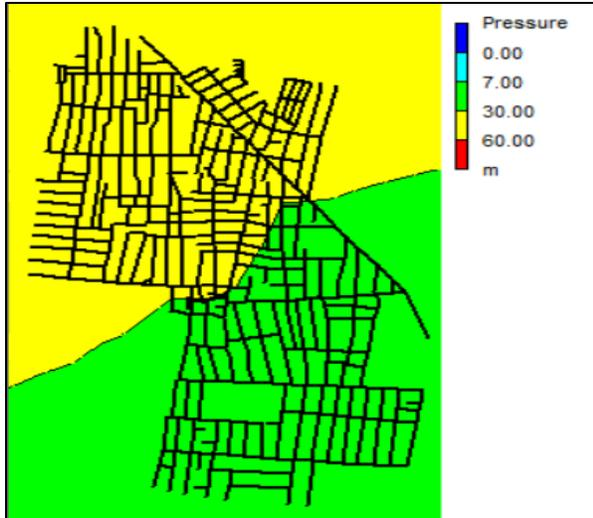
Figure 3: Contour Plot of Pressure of Water Distribution System for Srinagar Ward
