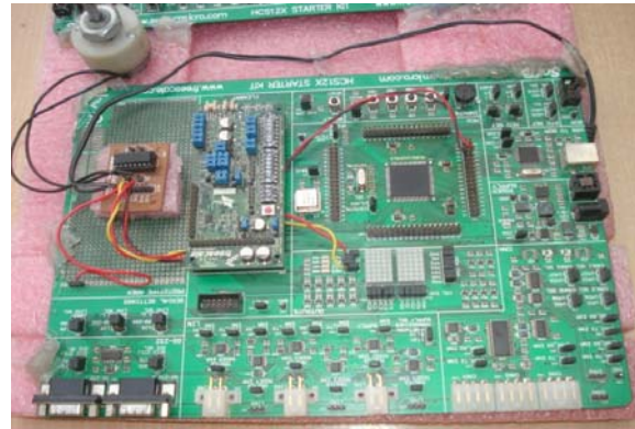
Fig. 10 : HCS12x Starter Kit configured as Power window node with DC motor
