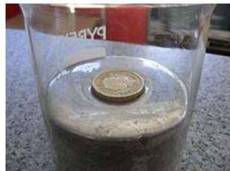
A coin density 7.6g/cc floats in mercury due to the combination of the buoyant force and surface tension.
